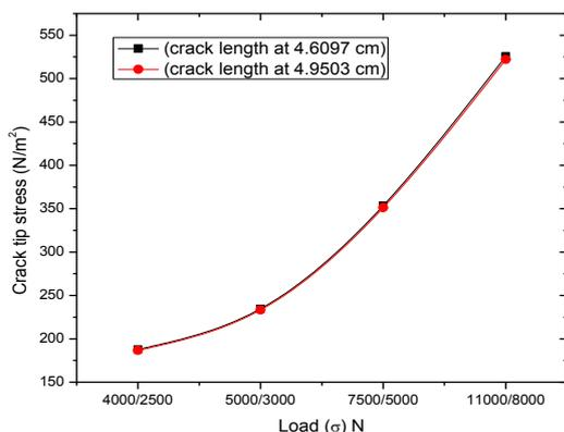
Figure 4.31 Load v/s crack Tip Stress
