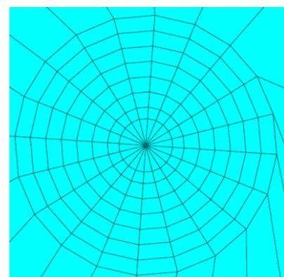
Figure 3.4 Enlarged view of crack tip
